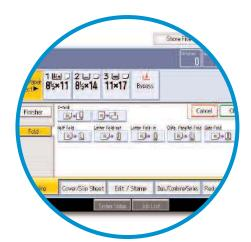
Choose from six different folding options, including Letter Fold (Tri-Fold) and Z-Fold, with the optional Multi-Fold Unit.
