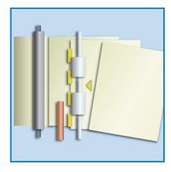
Mechanical paper registration automatically adjusts paper to ensure precise registration accuracy on the front and back of every sheet.
